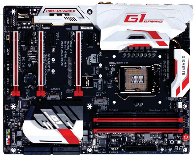
Gigabyte's Z170X-Gaming 7 supports simultaneous use of its CPU_FAN and CPU_OPT headers.
